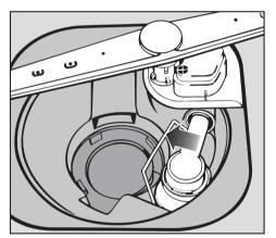
■ Tilt the locking clamp to the side and pull out the non-return valve.
